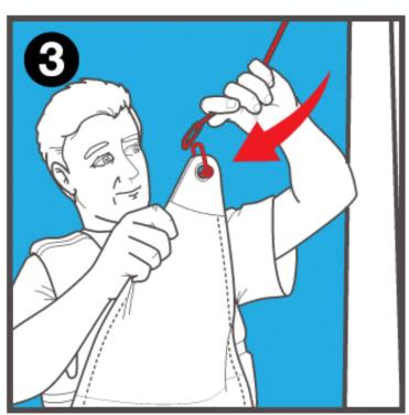
Attach the jib halyard to the head of the jib using a shackle.
