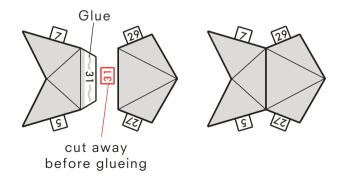
Note: Before glueing, cut away the number tab on the corresponding side.
